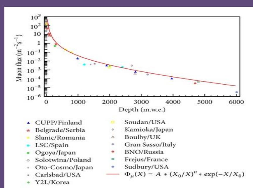
Muon Flux represented as a function of depth in various global locations. Graph is open access from Advances in High Energy Physics journal. Our expected data should show a similar correlation between depth and flux.
