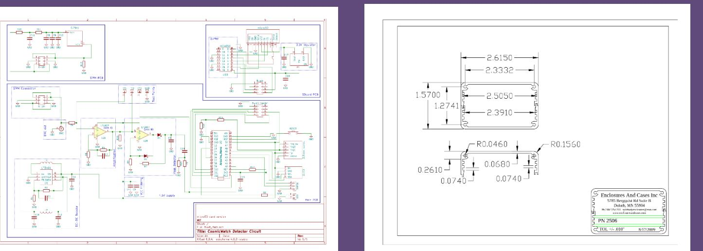
Cosmic watch circuit diagram (Left) and case dimensions (Right). All code, CAD files, and supporting information are available at <http://www.cosmicwatch.lns.mit.edu/detector>
