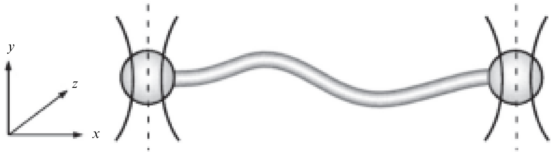
Fig 1: Experimental configuration to observe thermal force fluctuations in a DNA molecule using optical tweezers. Adapted from [1].
